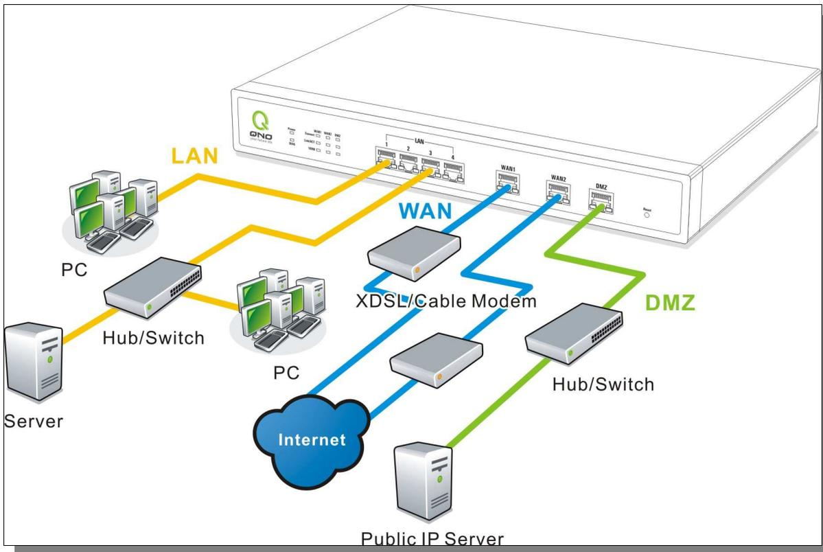
**WAN connection :** A WAN port can be connected with xDSL Modem, Fiber Modem, Switching Hub, or through an external router to connect to the Internet.
