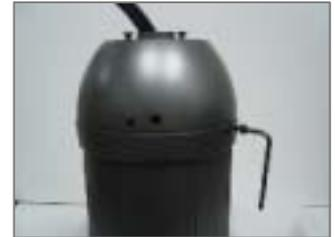
**Step 4** Get the ceiling mount bracket. Put cables into the tube, starting with the 9-pin alarm I/O (take the male part off to obtain smaller size). Have all connectors come out the tube from cable outlet near the top of the bracket.
