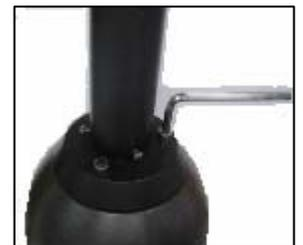
**Step 6** Mount the bracket onto ceiling and tight the bracket completely.
