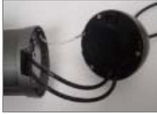
**Step 3** Fasten the sub-assembly and camera together at the joint of D-sub connectors. Rotate camera all the way in direction of clockwise. Fix the base to camera with the supplied screw and wrench.
