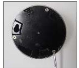
**Step 2** Hook the sub-assembly and camera with the safety cable located on the bottom of camera (left picture on below), then put the signal cables throughout the sub-assembly (right picture).
