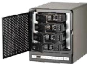
To ensure the data security, TS-409 offers advanced disk configurations for RAID 0, 1, 5, 6, 5 + Spare, Single, and JBOD.
