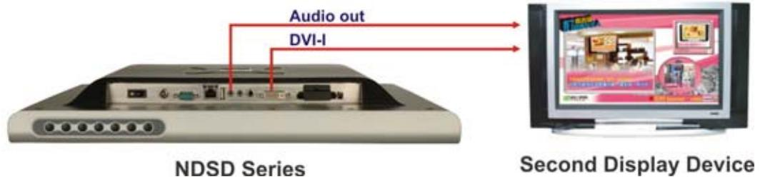
Figure 2-5: Second Display Device Connection
