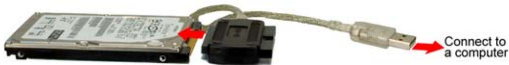
**Figure 2-1: Format the HDD via IDE-USB Cable**
