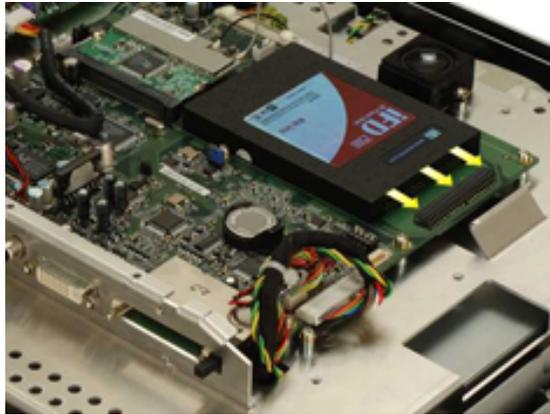
Figure 2-4: IDE HDD Installation
