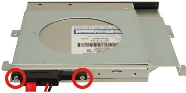
**Figure 8-17: SATA Cable Retention Screws**
