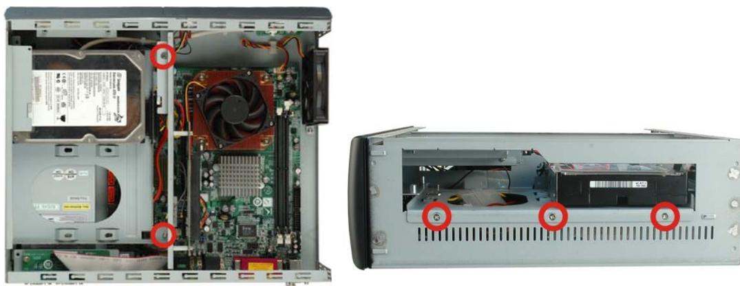
**Figure 8-7: HDD Bracket Retention Screws**
