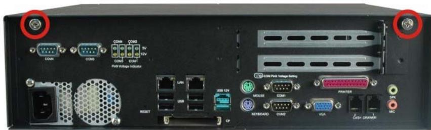
**Figure 8-1: Cover Case Thumb Screws**
