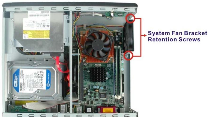
**Figure 8-5: System Fan Bracket Retention Screws**
