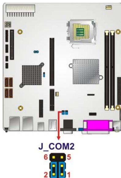
**Figure 3-6: COM 3/4 Pin 9 Setting Jumper Location**
