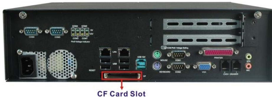
**Figure 4-1: CF Card Slot Cover Retention Screw**
