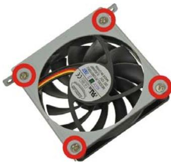
**Figure 8-6: System Fan Retention Screws**
