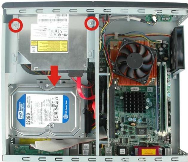
**Figure 8-16: ODD Bracket Retention Screws**
