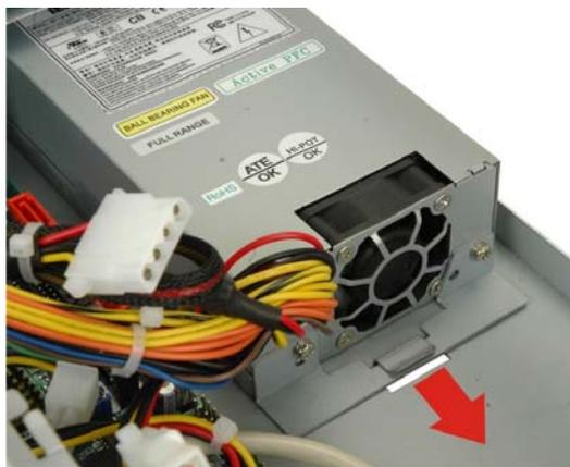
**Figure 8-13: Power Supply Removal**
