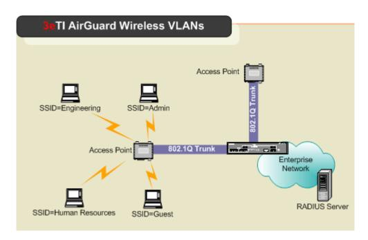
When VLAN is enabled, all data coming out of the WAN port is VLAN-tagged, which means an external network unit such as a router, switch, or a VLAN-enabled computer has to be used to terminate the VLAN traffic. Data originating from or targeting to a wireless network client is tagged with the VLAN ID corresponding to the SSID to which it is associated. Data generated by an Access Point itself is tagged with the management VLAN ID.
