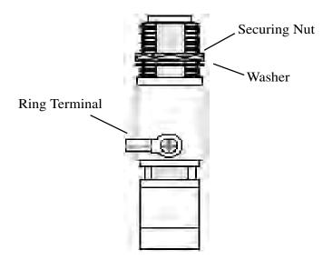
Attach the 10, 12, and 18-inch wires to the lightning arrestors ensuring that the smaller ring terminals and with identifying labels are used. Tighten the ring terminal securely using a screwdriver.
