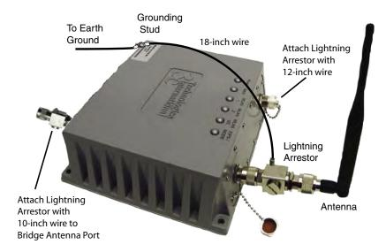
Attach the ring terminal from the Lightning Arrestors' ground cable to the grounding stud on the 3e–525C–3 unit. The lightning arrestor's ring terminal should be attached to the unit after the earth ground ring terminal is attached.
