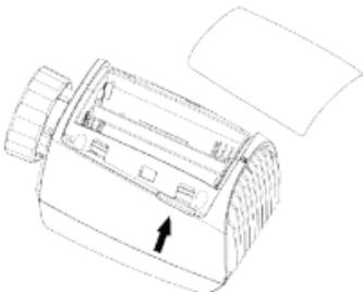
The service life of new alkaline batteries is approximately 1.5 years. A battery symbol (BAT) on the display indicates that the batteries need to be replaced. After removing the empty batteries, wait approx. 1 minute before inserting the new ones. This device does not support operation with rechargeable batteries.
